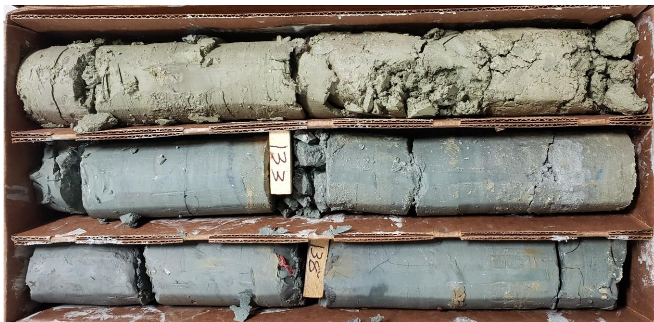
FIGURE 1 – Example of core from CVZ-71, the first hole drilled using PQ core. PQ-sized core has a larger diameter to provide more material for ongoing metallurgical testing. This particular section shows the transition from olive claystones to the blue reduced claystones. As a general rule, demonstrated by previous programs, the blue claystones tend to have higher lithium values.
