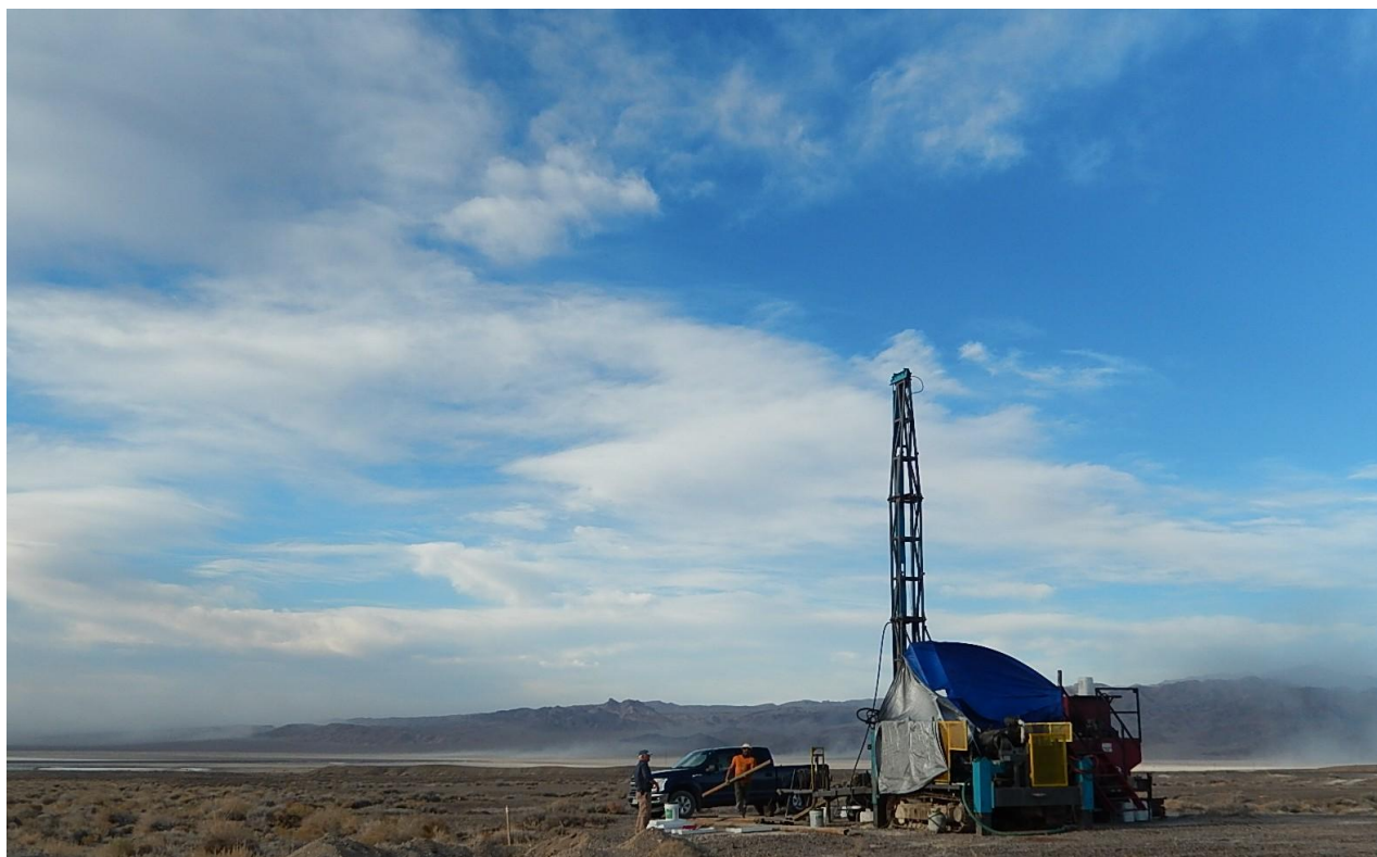
Figure 1 - LF-70 drill rig on CVZ-62 site, 2020-11-17, Brad Peek, Senior Geologist and Q.P. on site, looking northwest. CVZ-62 has 50 meters of lithium claystone and is continuing to drill in the claystones. Samples have been submitted to ALS laboratories for analysis.
