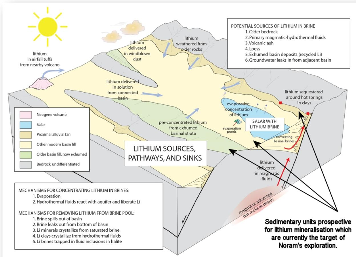
Figure 7.8 - Schematic deposit model for lithium brines (Bradley, 2013).
