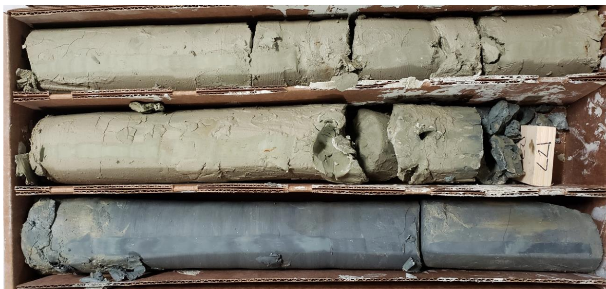
Figure 1. Example of core from CVZ-79; the interval from 124.0 to 129.5 ft (37.8 – 39.5 m). This particular section shows the transition from light olive claystones to the black reduced claystones. As a general rule, demonstrated by previous programs, the black claystones tend to have higher lithium values.
